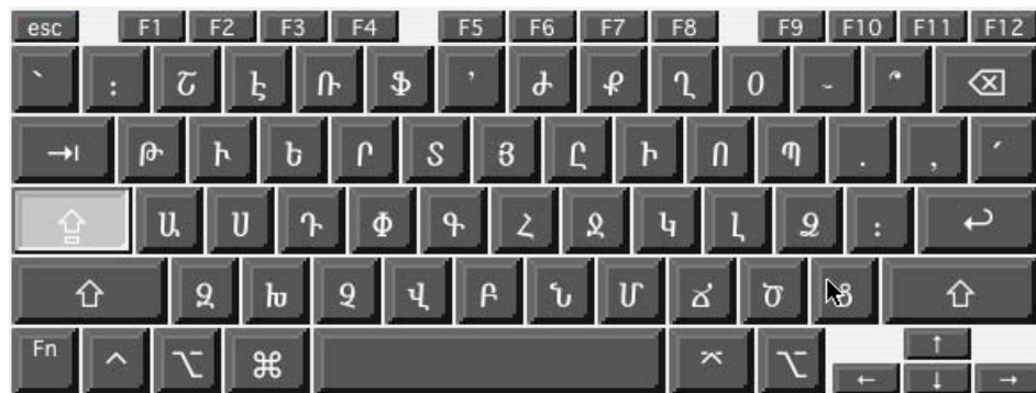
Figure 9. Armenian-RT keyboard layout. Both these keyboard layouts expose all Armenian characters without having to press the alt or option key. Both are free at telf.com.
